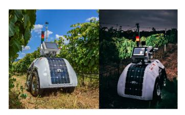
Autonomous vineyard monitoring robot works both day and night and features an Apogee infrared radiometer (SI-411).
